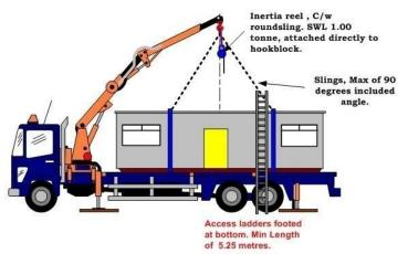
A second man must foot the ladder. The ladders must be in good order and free from any defects. The ladders must be long enough to reach the top of the cabin whilst on the truck. Do not access the cabin roof, rather, use ladder to access all 4 corners of the cabin to install the chain slings. Employ a full body harness and inertia and securely attached to the crane hook using a 1.00t sling.
